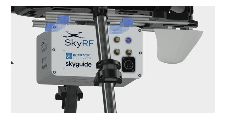
Connect the power supply and drone data interface to the transceiver. This is done by inserting the Neutrik NC10FXX-14-B connector. Connect the WIFI antenna.
